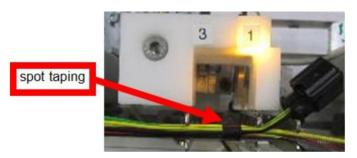
Figure 1.2. The spot taping procedure
