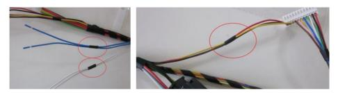
Figure 1.5. Spot typing process done by a worker
