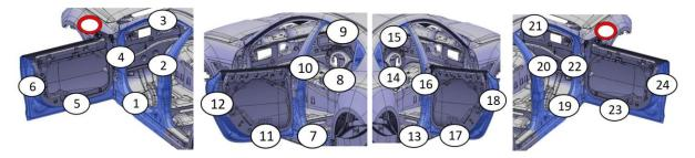
Figure 3.4. The predefined internal points to measure the thickness of the paint in 356 Sedan type cars
