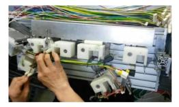
Figure 1.3. Assemble of wire harnesses and the spot taping process
