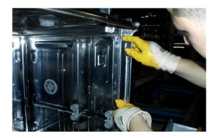
**Figure 2.5.** Assembling the gasket on the inner tube The current process can be seen in the <u>video</u>.
