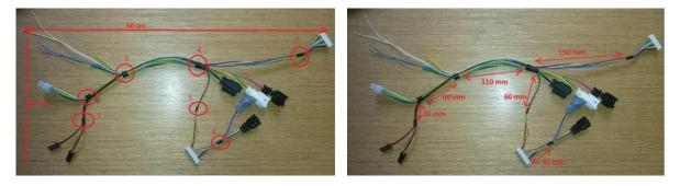
**Figure 1.6.** Cable assembly with marked taping spots and with dimensions between taping spots For spot taping, the taping pistol in Figure 1.7 is used.
