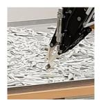
Figure 2.2. Grasping of the detected springs
