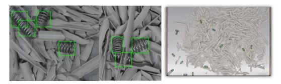
Figure 2.1. Visual detection of Magnox springs
